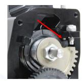
22) Reinstall the motor drive cover. Tighten the 4 screws securing the cover.
