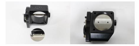
Apply red thread locker (Red Loctite) to the threads of the throttle plate screws. Install loosely.
