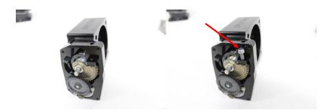
20) When closing the throttle plate by hand, you may notice that it "sticks" closed. To set the adjustment of this set screw, you will thread it in clockwise just until you can close the throttle by hand without it sticking. You want the throttle plate to seal as much as possible without it sticking closed. Once a position has been determined, hold the adjustment of the screw steady and then tighten the locking nut.
