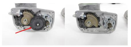
6) Remove the two screws securing the Drive motor. Remove the motor. Note: Use a small flat edge screw driver to pry the motor away from the housing. Working a small amount at a time and alternating sides. Do not bend the casing of the motor.
