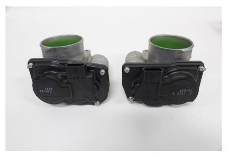
2) Remove the 4 screws per throttle body which secure the motor drive covers. EDIT? Note: T20 Security Torx
