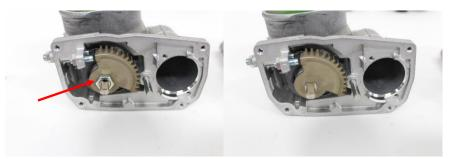
8) Remove the throttle shaft gear. Pay close attention when removing. This gear is under spring tension. Note how the tension is applied. Remove the spring underneath and set both to the side.
