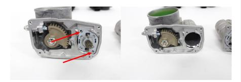
7) Remove the 12mm nut retaining the throttle shaft gear. Set to the side.
