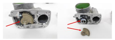
9) Remove the throttle stop cam. Pay close attention when removing. This stop cam is under spring tension. Note how the tension is applied. Remove the spring underneath and set both to the side.
