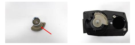
14) Install the drive motor using the two screws provided.
