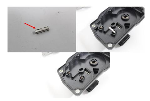
5) Remove the intermediate gear. Set to the side.
