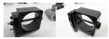
**13**) Install the throttle shaft gear and spring. Note the following pictures for orientation and position of the spring. The spring must sit in the detents shown in the pictures with the arrows.
