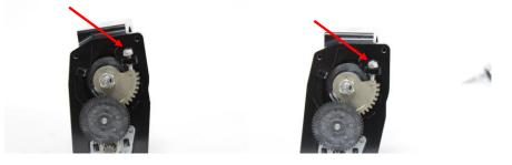
21) Now install the resting position set screw. This screw sets the resting throttle plate position. Important: The final position of this screw must be set by your tuner. To get a baseline, turn the screw in until it touches the stop cam or you feel the throttle plate just start to move from fully closed. Then Turn the screw 2 full revolutions clock-wise. Lock the screw down with the lock nut.
